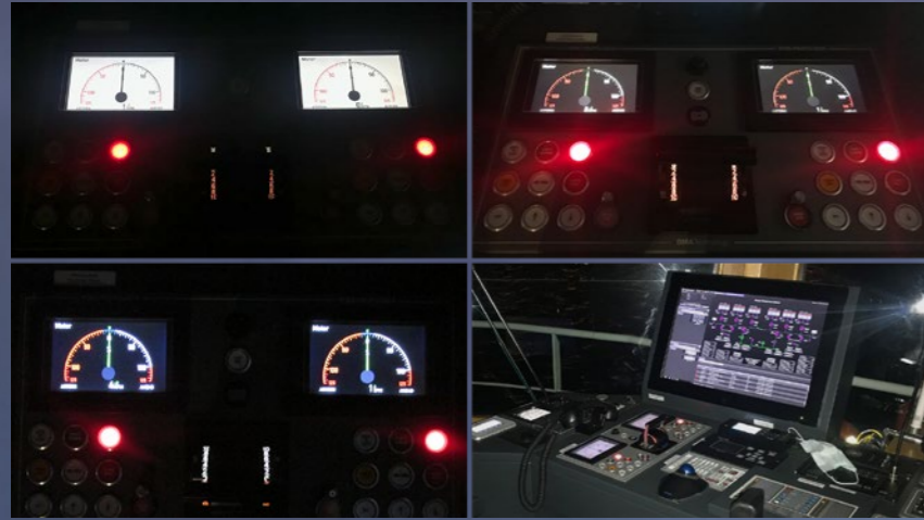
The customised XDi-N solution utilises the mode shift function, making it possible to shift between up to 4 predefined screens presenting combinations of relevant data.
